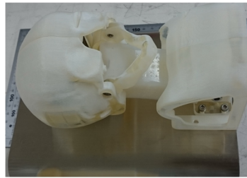
b. Internal structure of skeleton only. The temporomandibular joint is adjustable to the patient's preoperative condition.
