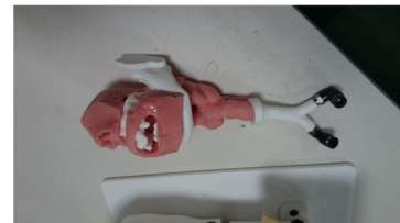
c. Oral and nasopharyngeal mucosa created with silicone rubber. Tracheal bifurcation and lung models are created. So, we can evaluate the mask ventilation is possible or not.
