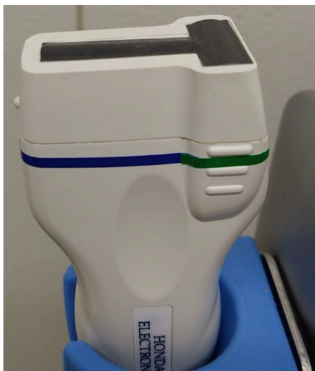
Fig. 1 A newly T-type probe (HLS-882, Honda Electronics Co., Ltd., Tokyo, Japan)
