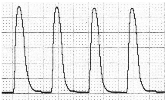
Figure 22.6. A control TOF. Four stimuli at 2 Hz (1 stimulus every 0.50 sec). The fourth response is 98% of the first, a TOF ratio of 0.98. Duration of each twitch response = approx. 300 \mu sec. This is a trace from a mechanomyographic recording.
