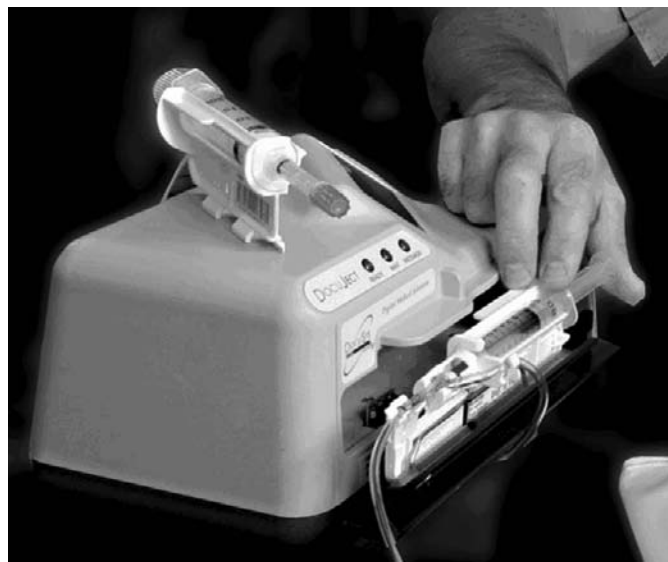
Figure 35.2. Anesthesia information management system (AIMS) medication scanning device – a device that verifies and records injections from barcoded medication syringes intended to reduce drug errors and improve documentation (Docuject, DocuSys, Mobile, AL).
