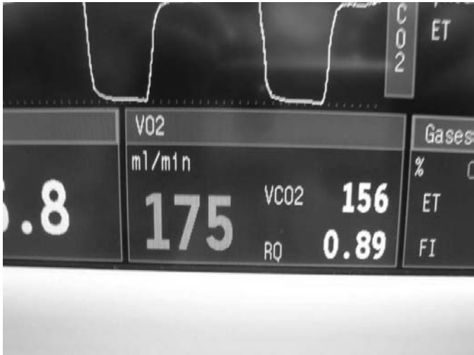
Figure 14.22. Screen of GE Datex-Ohmeda S5 Compact Airway Module monitor showing metabolic monitoring data (VO 2 , VCO 2 , RQ) from integrating concentration and flow signals.
