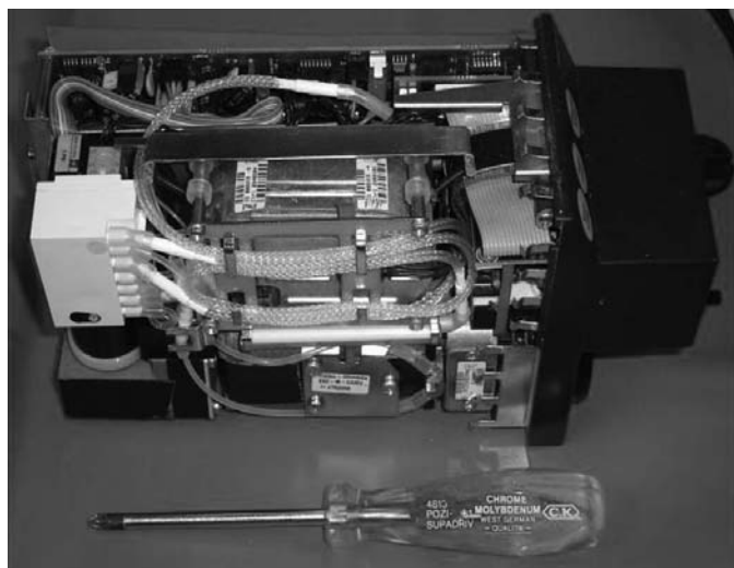
Figure 14.2. GE Compact Airway Module shown in Figure 14.1, opened to show miniaturization of gas monitoring technology.
