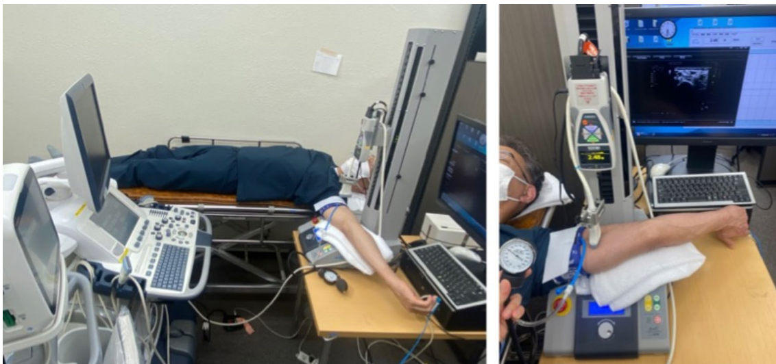
Fig. 2 The experimental system. Left: the entire system. An ultrasound probe was attached to a pressure-measuring device, and they were installed on a motorized table. The upper arm was tied at each tourniquet pressure and was placed under the device, and the pressure-measuring device was moved downward to compress the basilic
