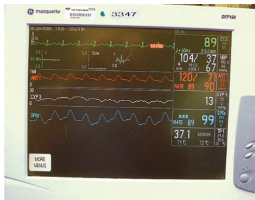
Figure 2.17 Integrated monitor displaying ECG and heart rate, non-invasive blood pressure (mmHg), arterial waveform and invasive blood pressure, central venous pressure (CVP) waveform, pulse oximeter waveform, saturation and temperature.
