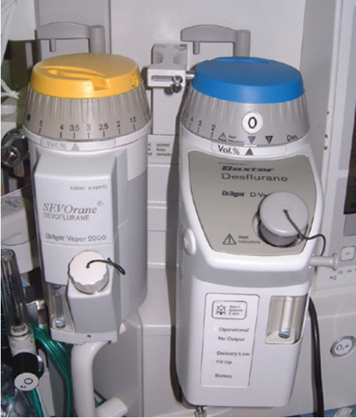
Figure 3.10 Sevoflurane vaporizer (left) and desflurane vaporizer (right) on an anaesthetic machine. Note the interlock positioned between the coloured dials to prevent simultaneous delivery of both vapours.
