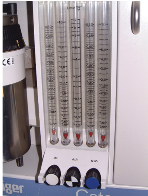
Figure 3.9 Oxygen, air and nitrous oxide flowmeters on an anaesthetic machine.
