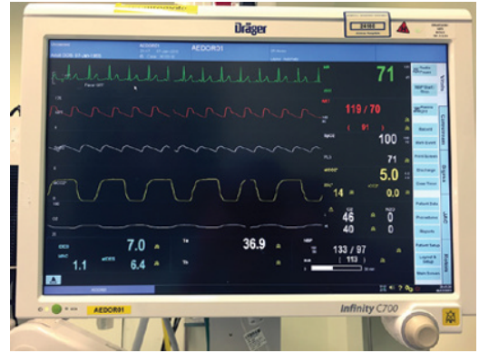
Figure 3.15 Integrated monitor displaying ECG and heart rate, invasive blood pressure (arterial waveform), pulse oximeter waveform, end-tidal carbon dioxide concentration and waveform, inspired and expired oxygen and desflurane concentrations, saturation and temperature.
