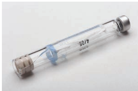
Figure 7-11. Cracked glass on dental cartridge.
