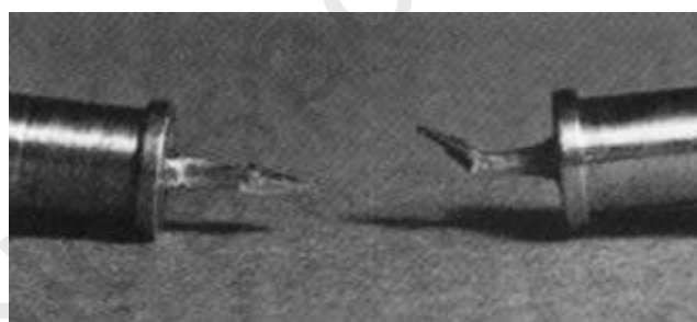
Figure 5-26. Note the bent harpoon of the syringe on the right.
