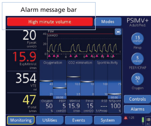
Fig. 12.3 The LCD screen of the HAMILTON-C2 ventilator. The alarm message bar is on the top left.
