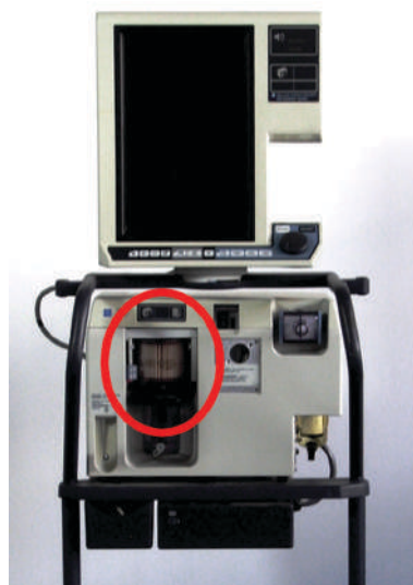
Fig. 6.13 Integrated heated filter in Puritan Bennett 840 ventilator.
