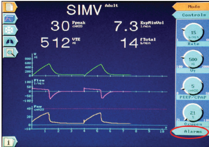
Fig. 12.6 The indicated arrow opens the alarm setting window in the GALILEO ventilator.
