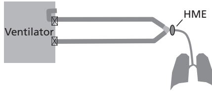
Fig. 6.18 Type D circuit with a heat and moisture exchanger (HME).
