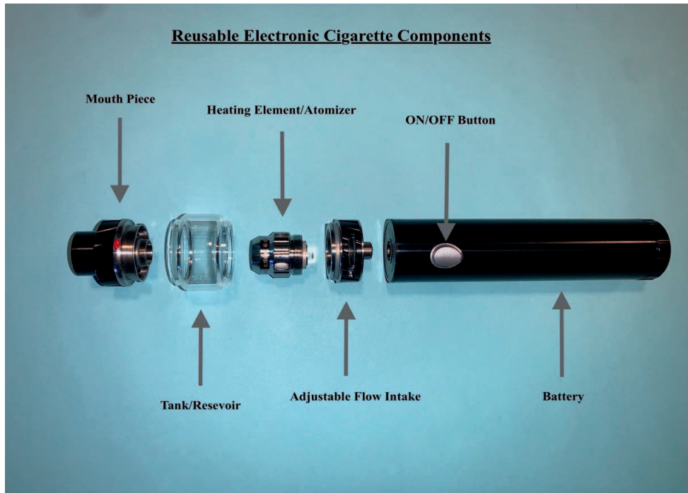
Figure 1. Reusable electronic cigarette components. Reusable e-cigarettes are composed of a plastic or glass tank which allows the user to store a greater volume of e-liquid. The heating element is typically an atomizer which allows for greater generation of aerosols. Reusable e-cigarettes contain a larger battery compared with disposable ones. A larger power supply to the heating element allows for a greater volume of aerosol to be generated with each puff.
