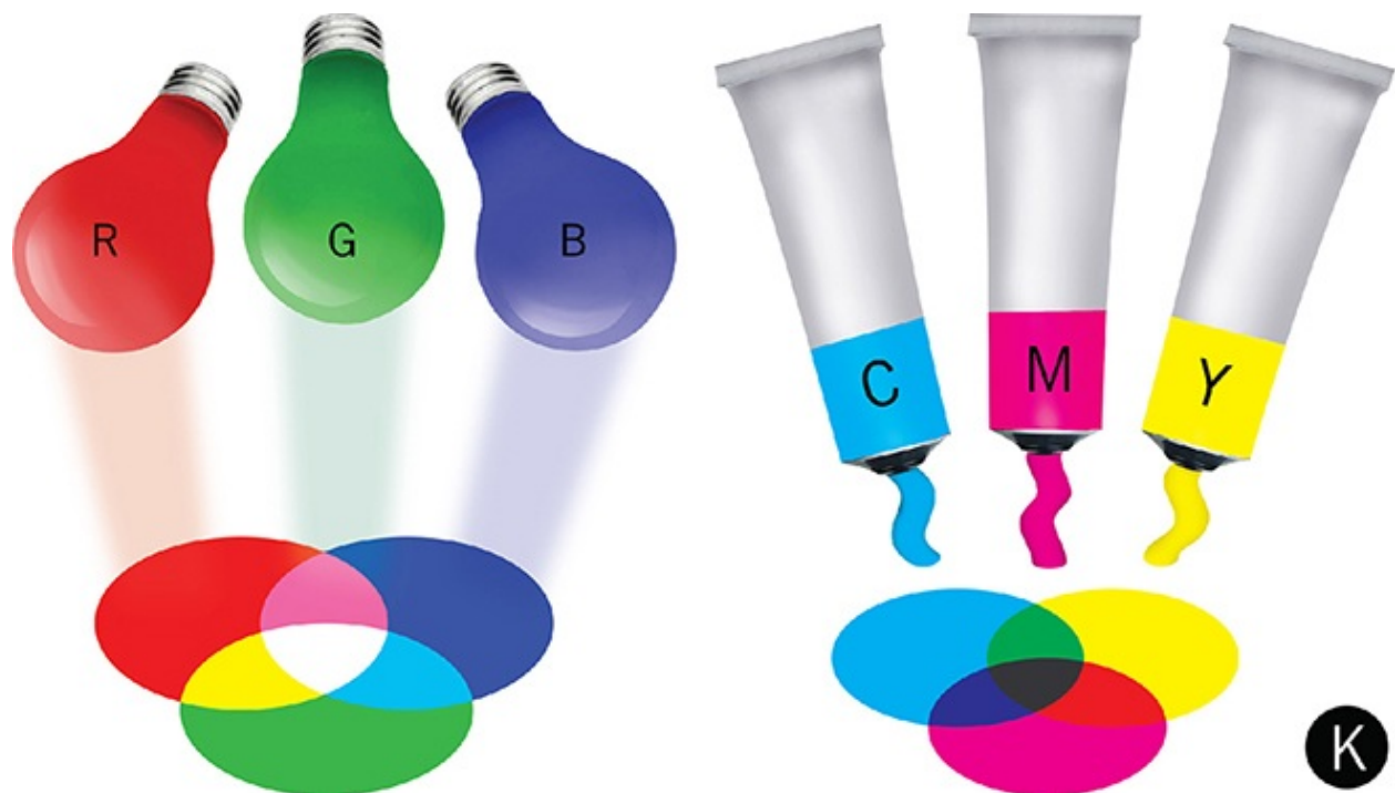
Figure 5.8 Color comes from light or pigment. The RGB color model is based on light. The CMYK color model is based on ink pigments. RGB is the color model used for communication design output to screen. CMYK is the color model used for communication design output to paper. Illustration by Kristen Crawford. Reproduced with kind permission of Kristen Crawford.
