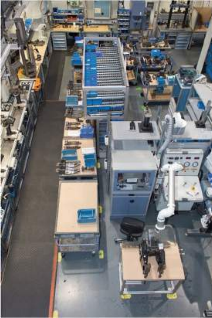
Fig. 10.6 Product—flow layout/assembly line for refurbishment processes [front view] (© Knorr-Bremse Berlin SFS GmbH)
