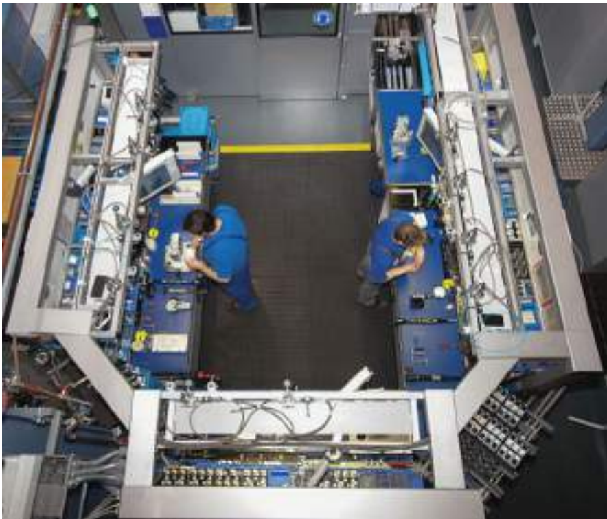
Fig. 10.9 Assembly of valves in a cell (© Knorr-Bremse Berlin SfS GmbH)
