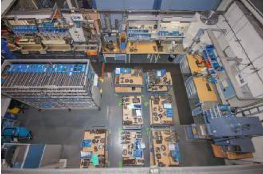
Fig. 10.7 Product—flow layout/assembly line for refurbishment processes [top view] (© Knorr-Bremse Berlin SFS GmbH)
