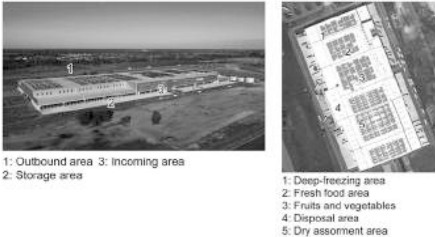
Fig. 10.12 Straightforward layout form of a warehouse
