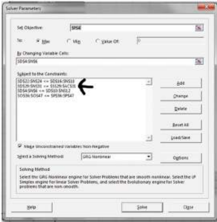
Fig. 17.15 Revised solver parameterization to achieve near-integer capacity allocation values: The labelled additional constraint is now considered while the solver processes the data
